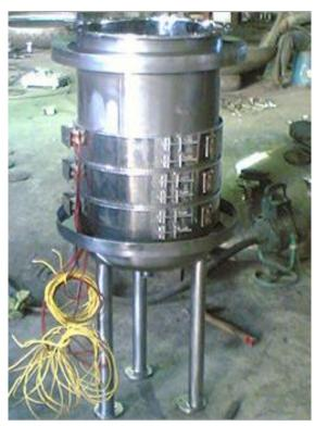
**Stainless Steel Tank with Band Heater System**
